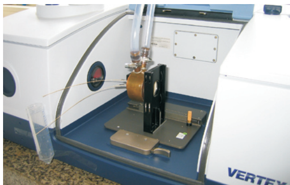
Fig. 9: Infrared transmission microcell for blood analysis
