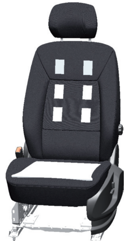
Fig. 4: Multichannel capacitive ECG system integrated into a driver seat.
