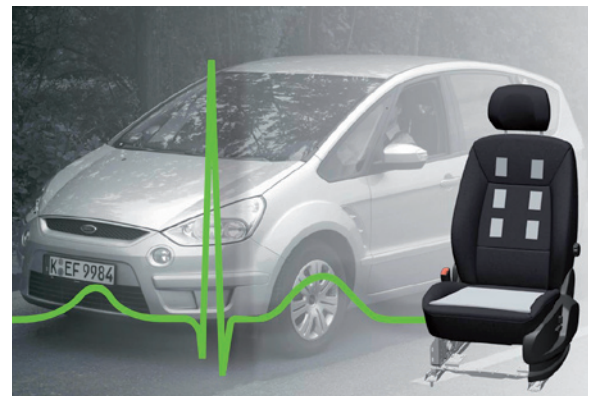
Fig. 4: Multichannel capacitive ECG system integrated into a driver seat.
