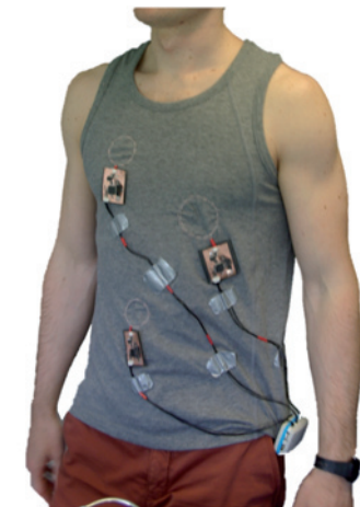
Fig. 7: Realization of a magnetic induction textile method integrated into T-shirt.
