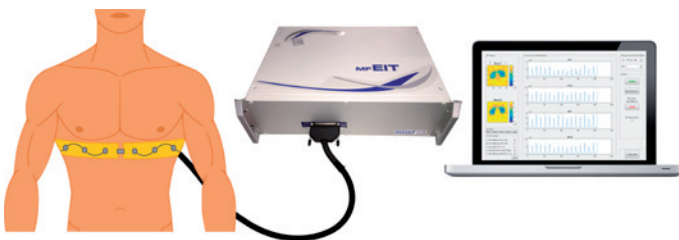
Fig. 9: System setup for multi-frequency electrical impedance tomography.
