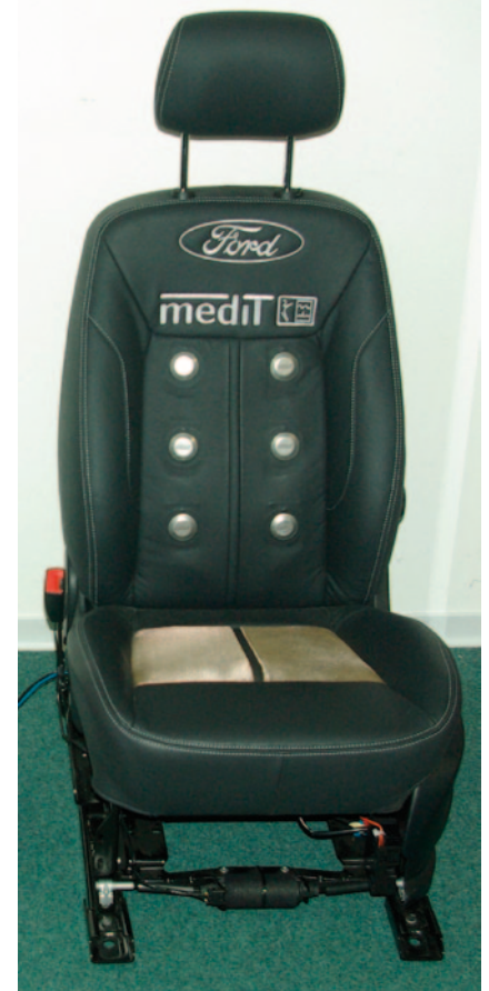
Fig. 9: Multi-channel cECGs integrated in a car seat.
